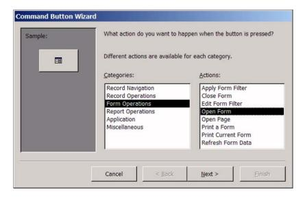
You need to select Form Operations, Open Form, ORDERS, "Open the form and find specific data to display", then match the relevant fields, type in some text for the button (perhaps 'Open Orders', although I have used 'GUI Button') and finally give it a name (which could also be 'Open Orders').
