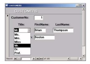
This combo box can be made to work in conjunction with, or independently of, the control applied at the table level.
