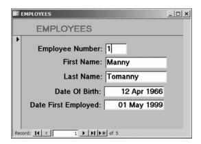
Some databases, such as Access, provide inbuilt tools for creating forms. Others, like Oracle, provide a separate tool (Oracle Forms which is a component of the Oracle Developer Suite) to build them. Forms can be produced as part of applications or as web pages (web forms). We'll drill into this later but for now you can think of forms as the user-friendly front end of the database.
